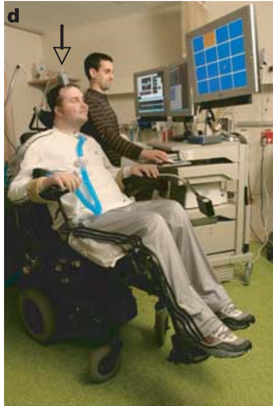
The first participant in the BrainGate trial (MN). The grey box (arrow) connected to the percutaneous pedestal contains amplifier and signal conditioning hardware; cabling brings the amplified neural signals to computers sitting beside the participant. He is looking at the monitor, directing the neural cursor towards the orange square in this 16-target 'grid' task. A technician appears (A.H.C.) behind the participant.
